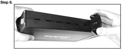
Place the Rubber Stands on the downside of the VPA-3528Net NetWork Storage, and position the Rubber Stand Location Positioner into the Rubber Stand Location Holes on the downside of the NetWork Storage.
